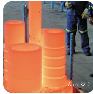
Vergüten, glühende Charge / tempering, red-hot batch
