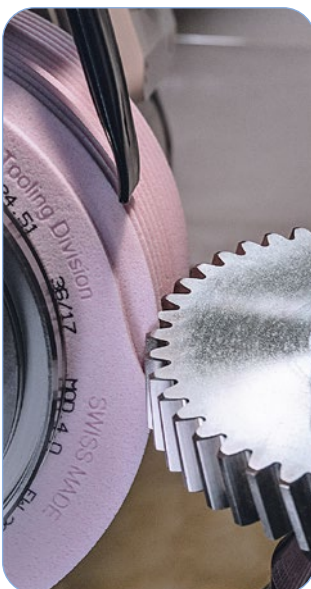
Wälzschleifmaschine / gear grinding machine
